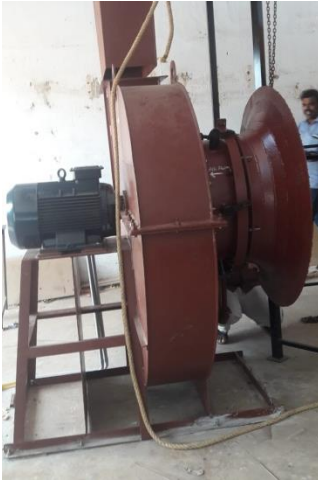
Fan design done and tested at NIT, Trichy Lab for Electro static Precipator Flow Model Testing as part of Consultancy projects
